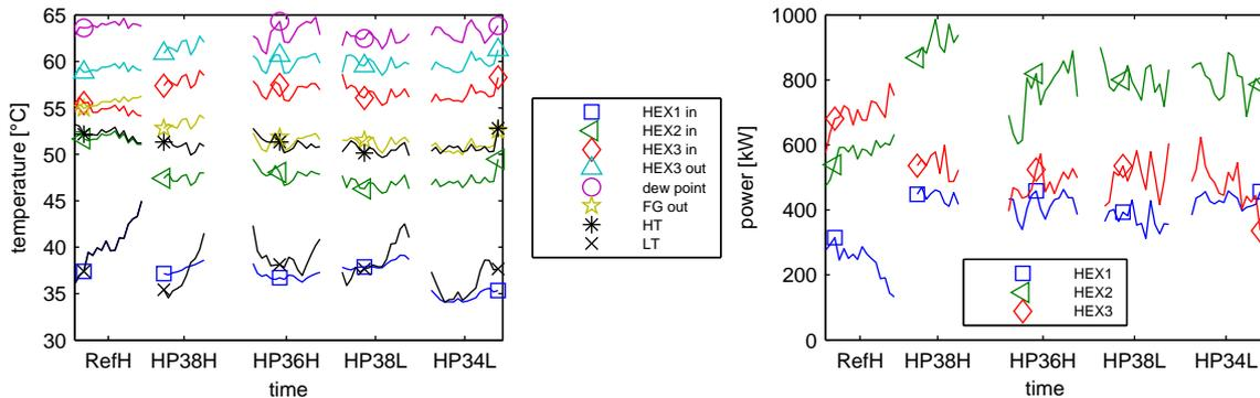
Figure 6: a) Temperatures in the condensing heat exchanger. b) Thermal power in the condensing heat exchanger.
