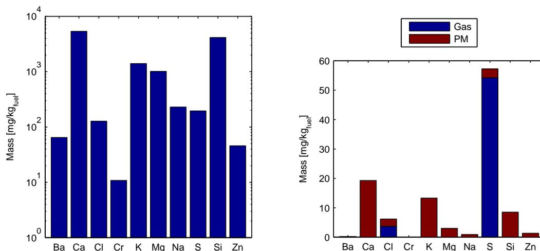
Figure 7: Mass balance of chemical elements. a) Total amount per kg fuel. b) Mass of chemical elements found in condensate from gaseous source (Gas) and from particulate matter (PM).
