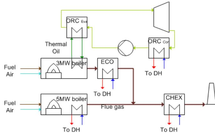
Figure 1: Simplified sketch of the plant. DH – district heating, ORC – Organic Rankine Cycle, CHEX – condensing heat exchanger, ECO – economizer.
