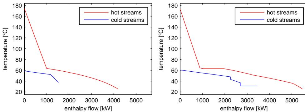
Figure 3: Pinch diagram of CHEX a) without heat pump; b) with heat pump.
