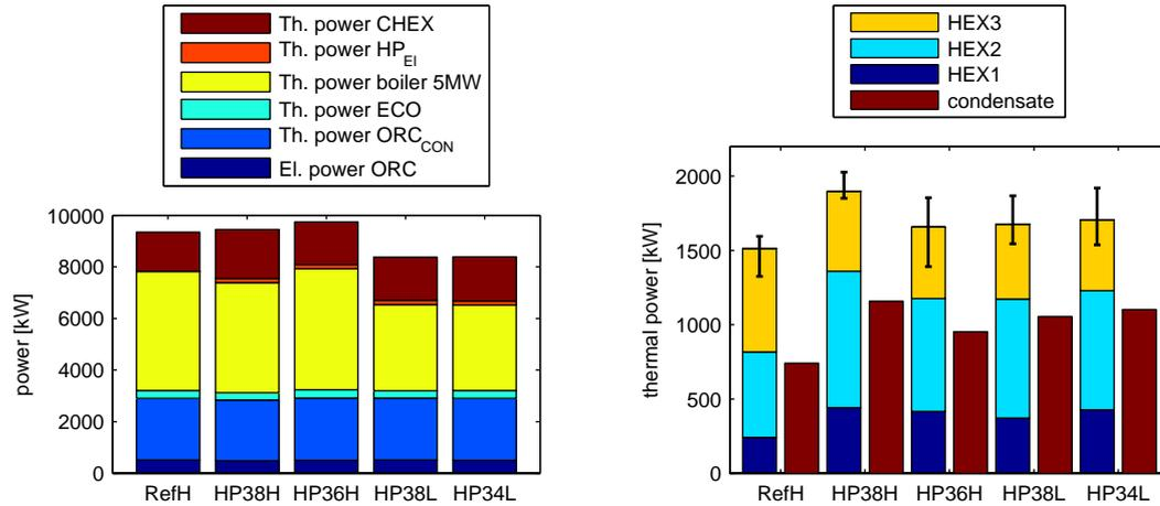
Figure 5: a) Thermal and electric power outputs of the plant. b) Thermal power in the bundle groups of the condensing heat exchanger (HEX1, HEX2 and HEX3) and thermal power associated with flue gas condensation.
