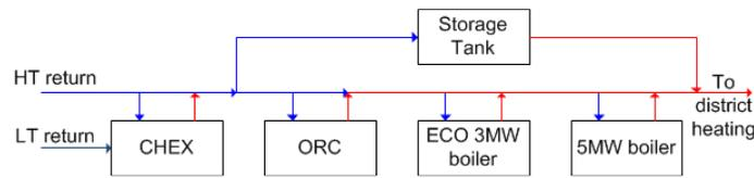
Figure 2: Sketch of the plant hydraulics. ORC – Organic Rankine Cycle, ECO – economizer
