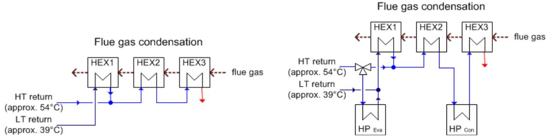
Figure 4: Sketch of the condensation system before (left) and after (right) the integration of the heat pump.
