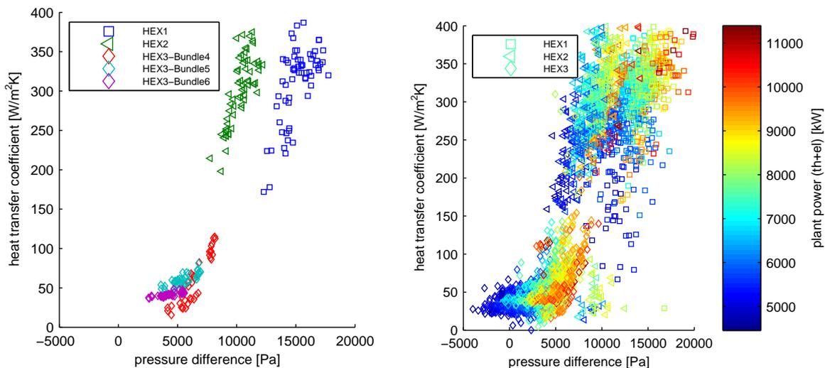
Figure 8: Heat transfer rate in the condensing heat exchanger vs. the approximated pressure difference driving the condensation. a) Data from operating points in Table 2. b) Data registered between 26.1.2014 and 5.2.2014, the colour indicates the plant power (thermal and electric outputs).
